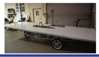
We also reconstructed the "wing" that holds the solar cells for TARS, our solar car, after we discovered flaws in our previous design. We have learned from our mistakes and have even been able to make our redesigned "wing" both stronger and lighter.
