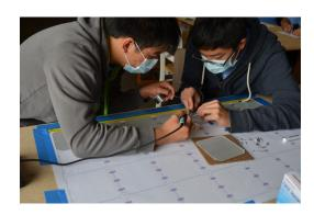
With the arrival of the shipment of our solar cells, we began a massive operation of taking every individual solar cell and connecting them to other each other to create 4x7 modules that will eventually be encapsulated and mounted on TARS. Due to the high efficiency of these cells, TARS will be competing in the Advanced Division of the Solar Car Challenge this summer.
