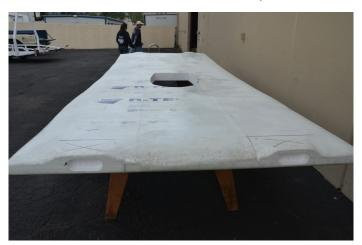
For TARS, we cut out holes in the array platform for our canopy and the brake and signal lights. Next, we plan to install the swing arm and motor. Although CASE is our current priority, we are working hard to have this car finished in the near future as well.
